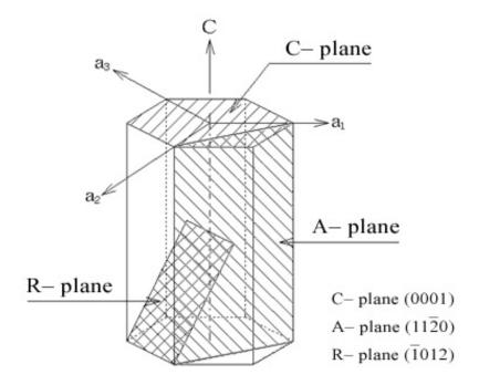
The structure of the primary planes of the sapphire crystal corresponding to the structure system of sapphire. Shown in this Figure, the C-plane is (0001), A-plane is (1120) and R-plane (1012)
